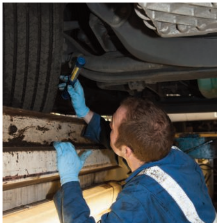
Check for signs of grease leaking from the axle bearings, and consider bearings and seals
