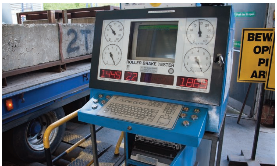
Trailers and semi-trailers should now complete at least three successful brake efficiency tests throughout the year, in addition to the annual MOT test: Guide to Maintaining Roadworthiness
