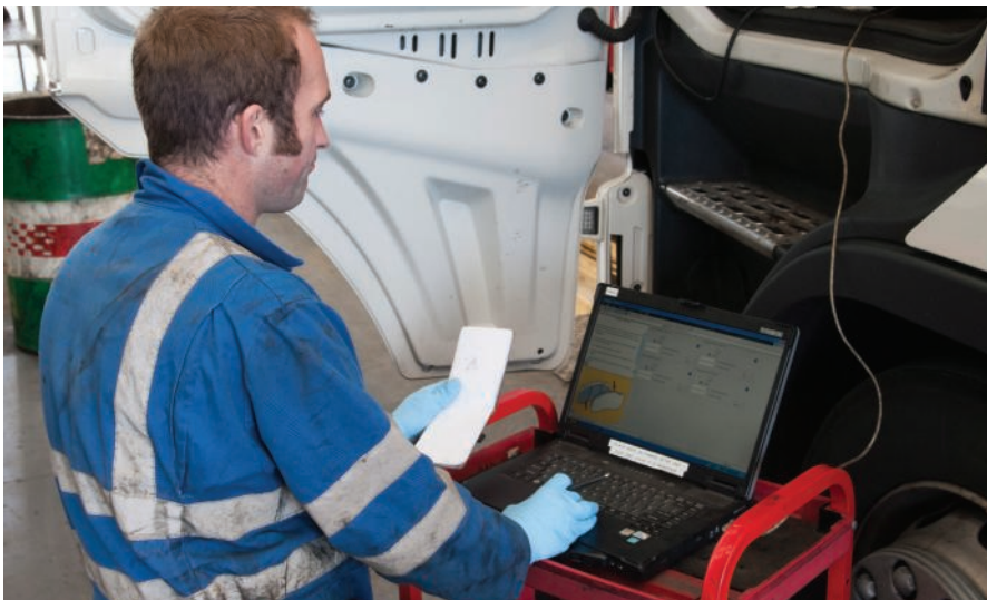
If the trailer is equipped with an information centre, use the diagnostic window to check for previous and current fault codes, and action accordingly
